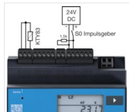
Fig.: Example thermistor input (KTY83) and S0 pulse generator
